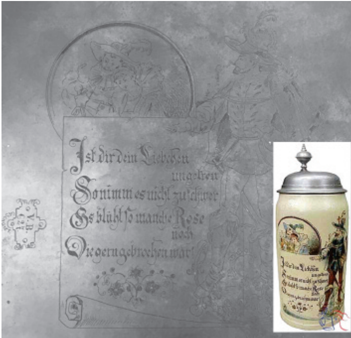
Figure 14- Engraved zinc printing plate for VBM stein 1526/627 (shown in inset)
