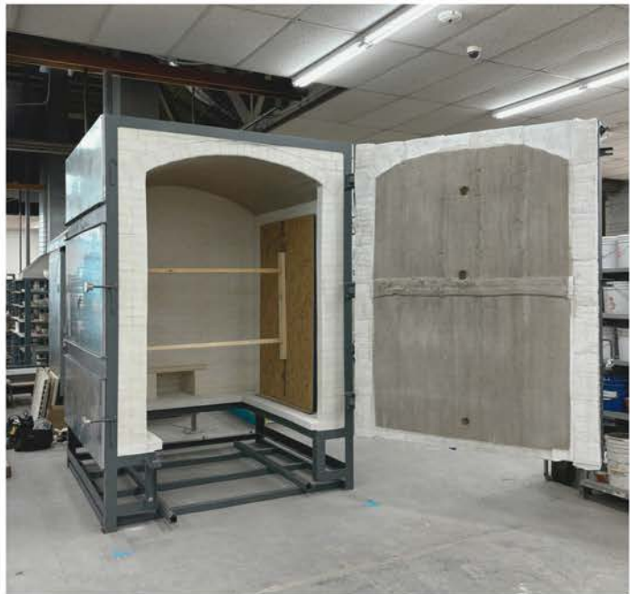
The kiln in place, ready to be hooked up to gas and exhaust
